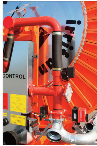
Automatic shut-off valve VA
