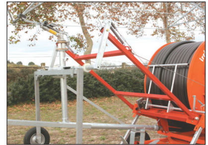
Automatic trolley hooking
