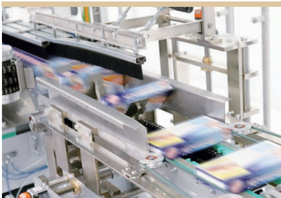
Product erection with a paddle chain
