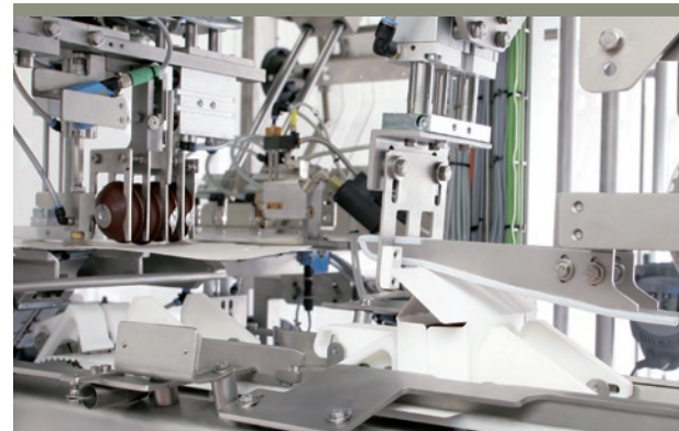
Transfer of the hot chocolate capsules onto the cardboard blank and subsequent folding of the blank around the product formation
