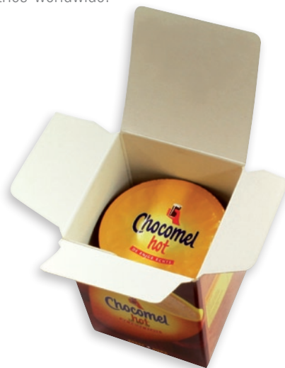
Transfer of the hot chocolate capsules onto the cardboard blank and subsequent folding of the blank around the product formation
