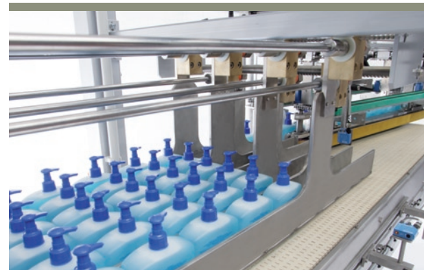
Single lane product infeed and distribution into the lanes via a lane belt divider
