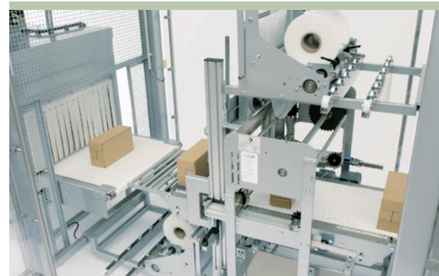
Transport of the finished wrap-around cases through the film section with shrink tunnel
