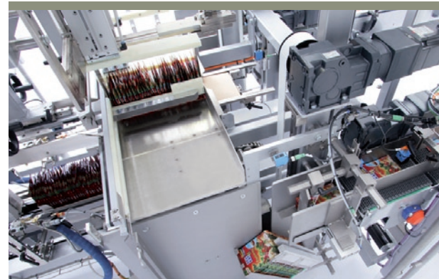
Pivoting stacking shaft transports the pouches directly onto the tray blank
