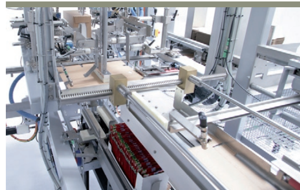
Lid forming station with lid waiting to be suctioned up into the forming tool
