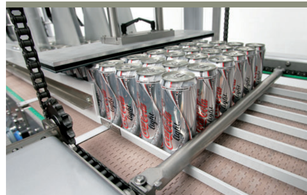
Infed and subsequent grouping of 0.33 liter beverage cans
