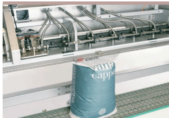
Heating section for inner-liner sealing
