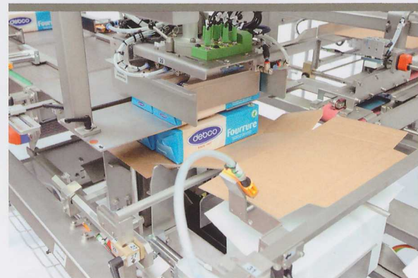
Controlled transfer of two margarine blocks onto the wrap-around blank or respectively onto the first layer by stacking
