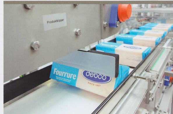
Feeding in and turning products 90° at the inflow of the VP 451
