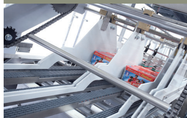
Infeed and grouping of Meadpacks in the VP 540
