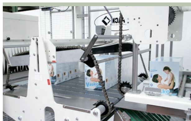
Wrapping products with the film wrapper and subsequent transport into the shrink tunnel
