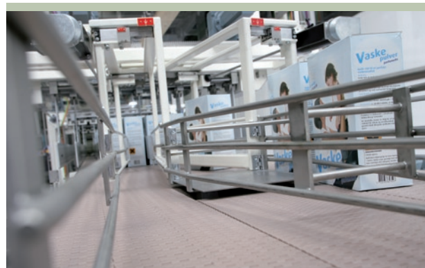
Fully automatic lane dividing system of the SW 90 M-40
