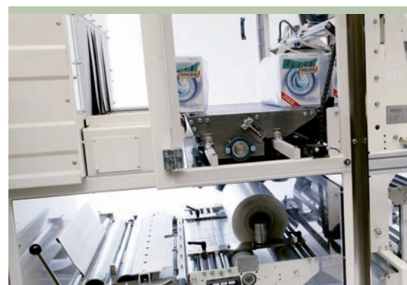
Side view film feed and film wrapping station
