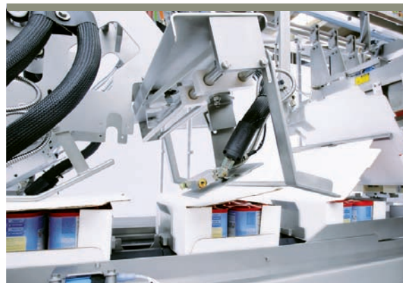
Product transport on the index chain through the machine
