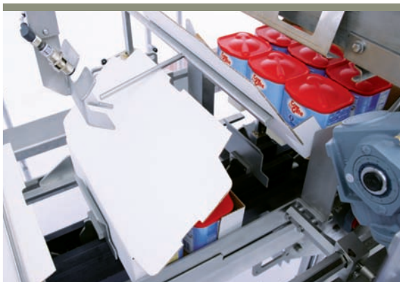
Servo-driven lowering principle
