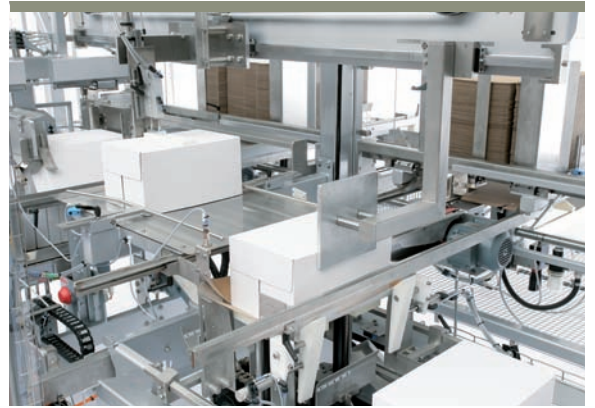
Lowering into the tray
