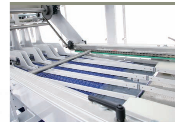
Overhead chain product transport and track chains after grouping station
