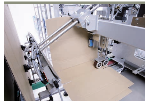
Blank uptake and positioning in standard magazine "Wrap-around"
