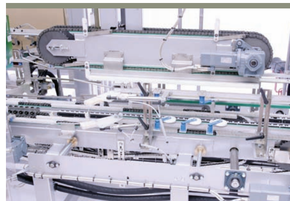
Pressing channel with side guides and upper pressing chain
