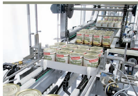
Tray transport chain and glueing station
